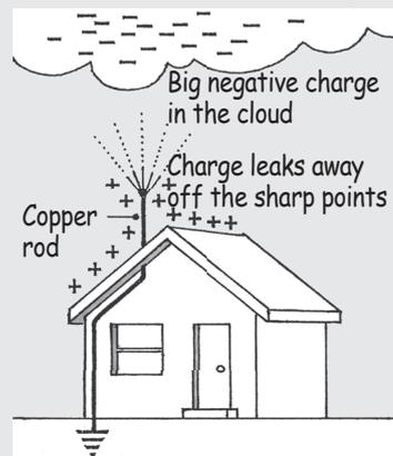
**Figure 24:** Electric charge flows over the outside of a metal shape.
