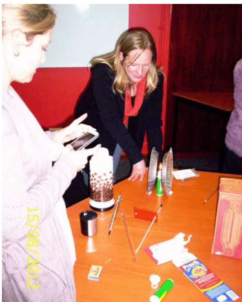
Cathy Linnell setting up a simple demo apparatus; it shows that black surfaces absorb radiated energy more quickly than silver, shiny surfaces.
