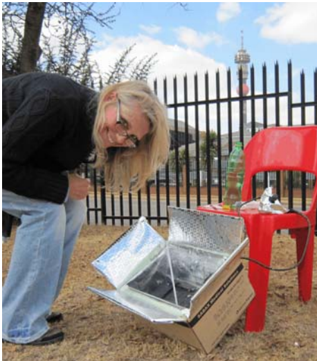
Mandy fitting a thermometer to the solar water-heater. It went to 107 °C
